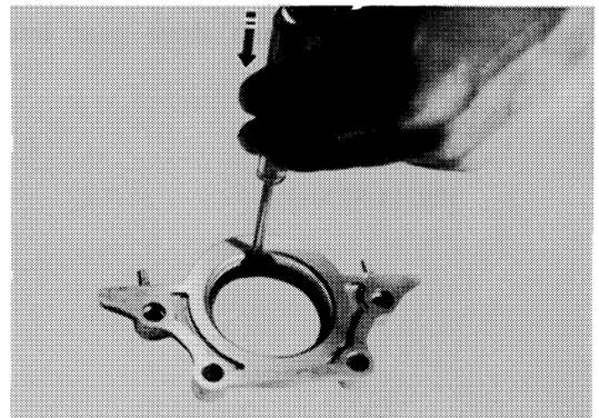
2. Install a new front oil seal using a drift that will catch the seals outer diameter and drive it squarely into the seal's boss.
